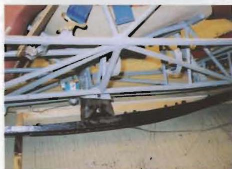
Top left: the nosewheel, a modification signed off in June 1985, will absorb impact energy but also cause rebound Left: the skid's rubber mounting block, directly under the front seatpan, will transmit impact loads up the spine Above: Les Neil releases the suspended ASK-13 (popularly known as a "K-13") for one of the series of tests
