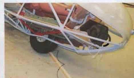
After the final, 2ft drop: note the deformed longeron. This was after being subjected to loads well beyond what the aircraft would be designed to withstand without structural damage (Tony Segal)
