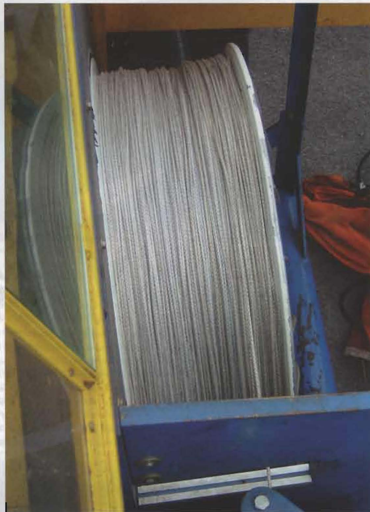
Right: A drum of the rope fitted to the club's homebuilt TOST winch
