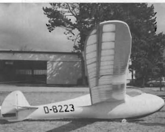
Below: Transparent fabric on the high-aspect ratio wing
