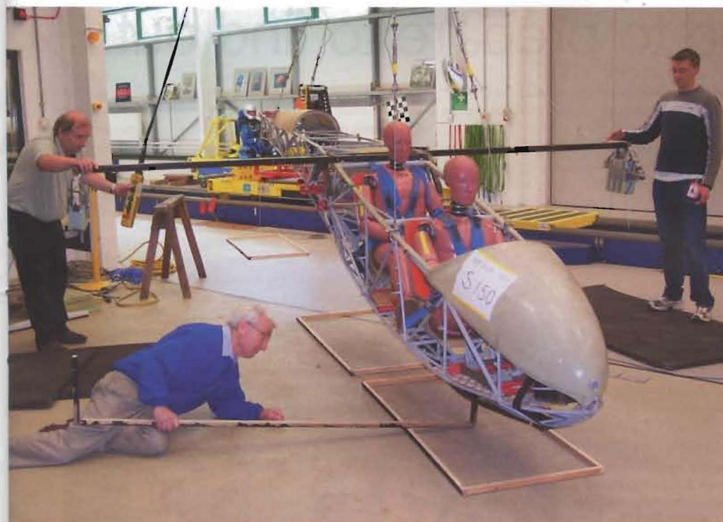
Above, from left: Les Neil, a Senior Consultant Engineer at the Centre for Human Sciences, QinetiQ, Tony Segal and Luke Cooper-Berry, of Imperial College, prepare for a test. Tony is measuring the height of the drop.
