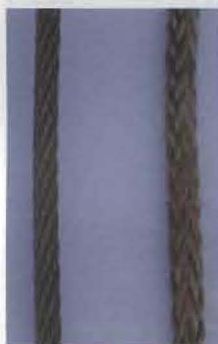
Above: Plasma rope compared to 5mm steel cable (on the left). The rope develops a slightly furry outer layer after being used for a while. This protects the rope and inhibits further wear. Bannerdown runs the rope along a tarmac runway, although this hasn't appeared to cause wear problems, mainly because it is so light.
