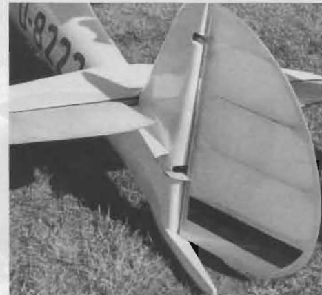
Below: A small rudder, hinged slightly forward of the fin
